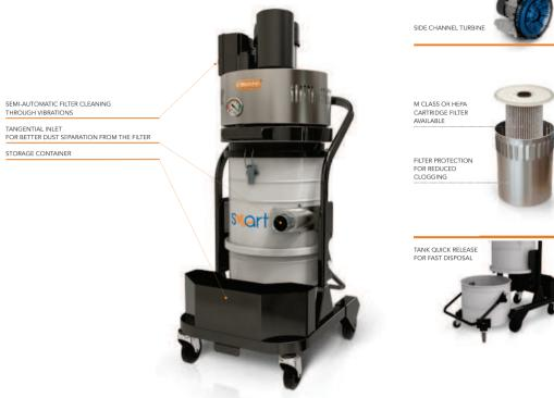
SMART 350 D is a single-phase industrial vacuum cleaner to 3 motors, the ideal model to be entrusted with any kind of general cleaning of the company. Its maneuverability, combined with compactness, allows easy movement even in the most confined spaces facilitating routine cleaning of the machine or the industrial environments. Due to its effectiveness the time required for cleaning are reduced, benefiting in terms of time and costs.
