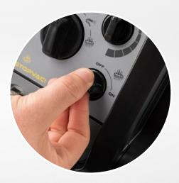
ON: NONSTOPVAC! is activated OFF: NONSTOPVAC! is deactivated.
