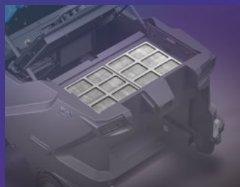
Carpet floor pre-filter for capturing fluff
